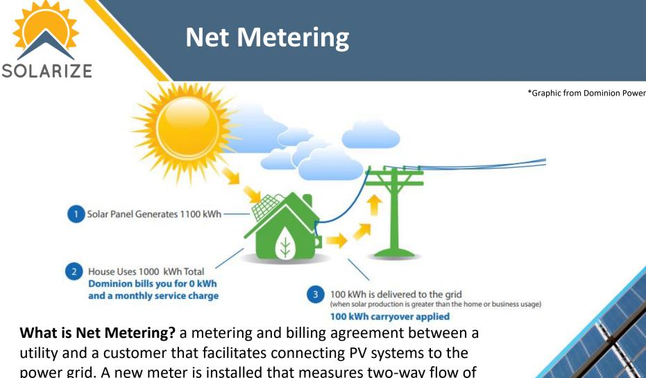
What is Net Metering? a metering and billing agreement between a utility and a customer that facilitates connecting PV systems to the power grid. A new meter is installed that measures two-way flow of electricity. The energy your system makes is first used on site. When your solar system is making more electricity than you are using at the time, the excess electricity is recorded by the meter as it flows back into the grid and is credited against future electricity use.
